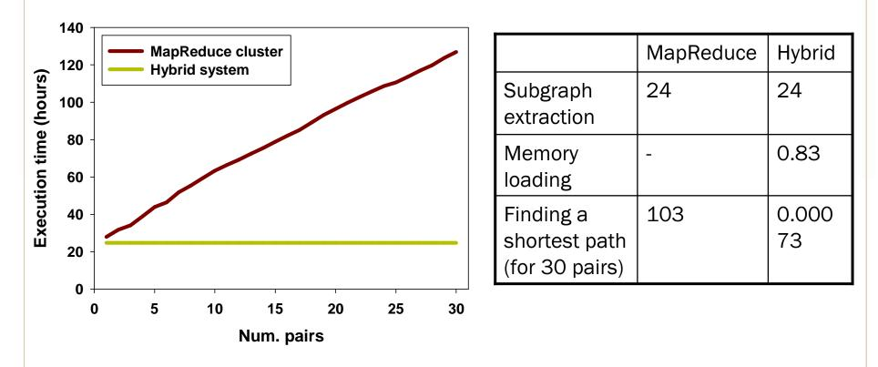
Once the subgraph is loaded into the memory, the hybrid system analyzes the subgraph five orders of magnitude faster than the MapReduce cluster (103 hours vs 2.6 seconds).
