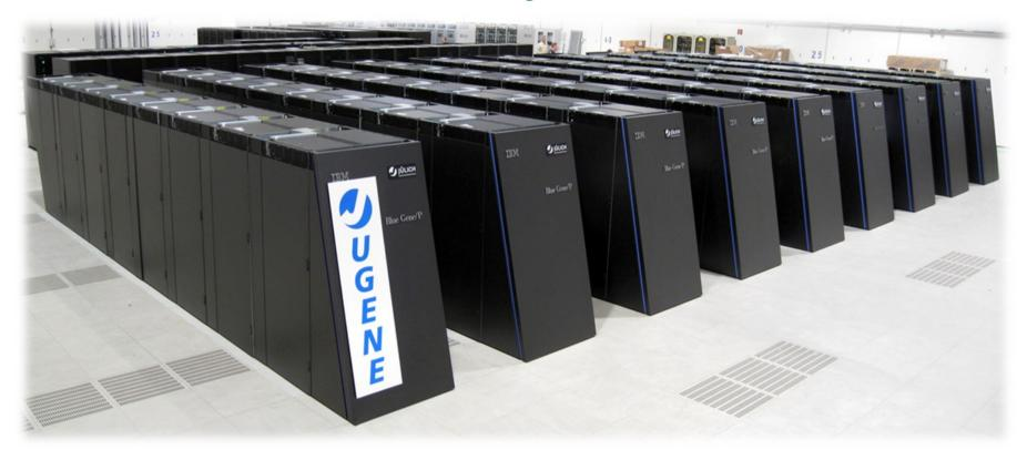
72 racks with 32 nodecards of 32 compute nodes (multiple networks)
